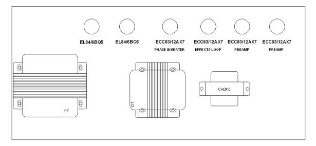
The Intruder uses four ECC83/12AX7 tubes and two 6BQ5/EL84 output tubes (or two EL34 tubes in the 30W or 50W version). The preamp tube function is as follows, starting at the side closest to the input jack: preamp 1 (ECC83/12AX7), preamp 2/cathode follower (ECC83/12AX7), effects loop driver/receiver (ECC83/12AX7), and phase inverter(ECC83/12AX7). The chassis top view layout is shown in the diagram above.
