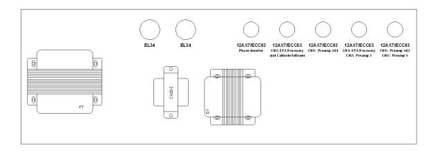
The Sabre uses five 12AX7/ECC83 tubes and EL34. The preamp tube function is as follows, starting at the side closest to the input jack: CH1 preamp 1/CH2 preamp 1 (12AX7/ECC83), CH1 effects recovery amp/CH2 preamp 2 (12AX7/ECC83), CH2 preamp 3/CH2 preamp 4 (12AX7/ECC83), CH2 effects recovery amp/CH2 cathode follower (12AX7/ECC83), and phase inverter(12AX7/ECC83). The chassis top view layout is shown in the diagram above.
